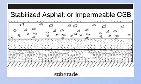
▶ Depends on thickness of flexible layer on top of old PCC – can use premium HMA on top and lower stabilized layers with recycled HMA, PCC and CSB. Need to be careful to avoid trapped water with "sandwich" construction.
